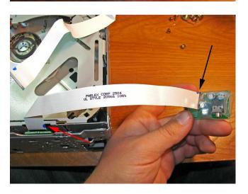
Insert the other end of the ribbon cable into the center plug on the aux-in board, with the orientation of the ribbon cable and board as shown in the image.
