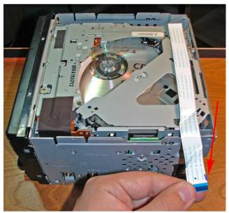
Straighten the cable and verify the correct side is marked.
