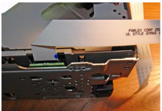
Plug the cable into the radio as shown - note the side of the cable with text showing.
