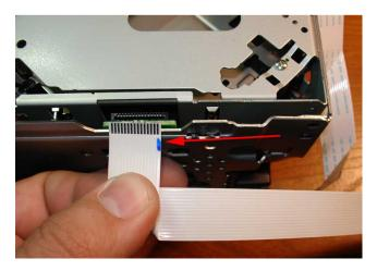
With the metal contacts of the ribbon cable facing up, mark the same side on the 8" ribbon cable provided on **both ends** to help identify the matching pin on each end.
