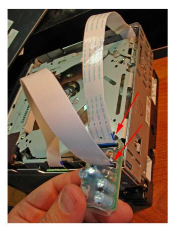
Plug the ribbon cable from the radio into the board as shown - the marked edges of the two ribbon cables should match and the orientation of the ribbon cables should look as it does in the image to the left.
