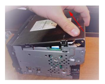
After the screws are removed, take off the top lid by lifting at the pry points indicated on the radio.
