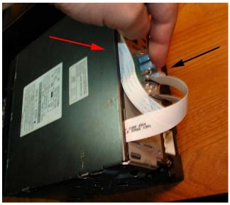
Reinstall the cover on the top of the radio and attach the board to the back of the radio with the Velcro supplied.
