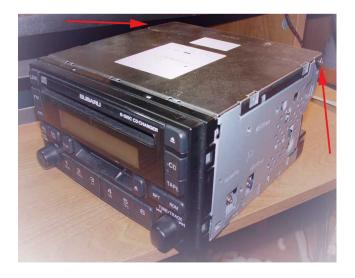
Next, remove the two screws at the back of the radio on the top cover.
