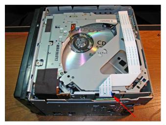
Mark the side of the ribbon cable where indicated to aid in installation of the board, then unplug the cable.
