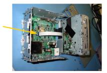
Before removing the CD changer completely, its ribbon cable needs to be disconnected from the radio. Gently pull it straight out from the connector.
