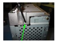
After the heat sink is removed, remove the top lid of the radio by taking out the two screws holding it in place and pop it off by lifting at the pry points indicated on the radio.
