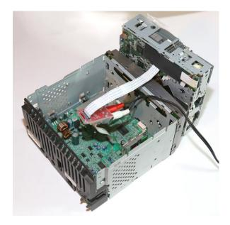
Once the patch cord is prepared, set the radio & changer + board next to each other. Plug the stereo patch cable into the aux port on the accessory board. The audio cable should insert completely into the jack on the aux board, clicking securely into place. Next plug the 4" ribbon cable into the connector on the radio that the CD
