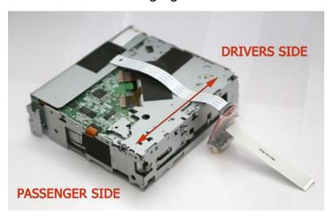
Next, route the stereo patch cord through the back of the radio. There is not a lot of room for this, so a thin audio cable is definitely a plus.
