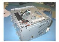
Once the heatsink and faceplate have been removed, 2 screws are left holding the CD changer in place. They are in the middle of the radio face as indicated with arrows in the picture. Once these are removed, the CD changer should lift out fairly easily. It may be necessary to gently pull on the sides at the back to free the mounting clips of the changer.
