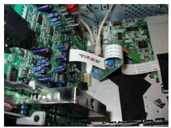
Once the patch cord is prepared, set the radio & changer + board next to each other. Plug the stereo patch cable into the aux port on the accessory board. The audio cable should insert completely into the jack on the aux board, clicking securely into place. Next plug the 2" ribbon cable into the connector on the radio that the CD changer ribbon was removed from earlier. Again, make sure all the ribbon cables are not twisted and the aux port is facing the passenger side of the radio.
