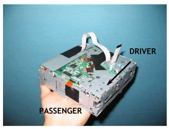
Next, route the stereo patch cord through the back of the radio. There is not a lot of room for this, so a thin audio cable is definitely a plus.
