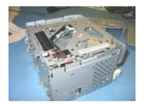
Once the heatsink and faceplate have been removed, 2 screws are left holding the CD changer in place. They are in the middle of the radio face as indicated with arrows in the picture. Once these are removed, the CD changer should lift out fairly easily. It may be necessary to gently pull on the sides at the back to free the mounting clips of the changer.
