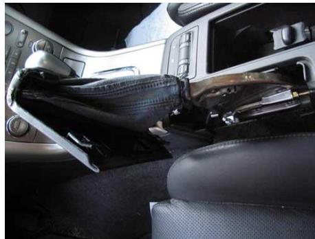
Next, empty the contents of the armrest cubby and remove the carpet on the bottom of the cubby to reveal two mounting screws. Removing these screws will loosen the rear of the armrest, and then only two plastic clips hold the front. Firmly grasping both sides of the front of the armrest and tugging straight up should dislodge both of these clips. It's unnecessary to completely remove the armrest, simply move it back a few inches to better reveal the transmission mount trim.
