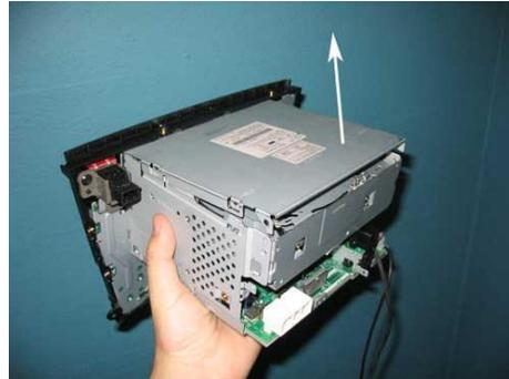
The next step is to remove the face of the radio. Several screws hold it in place including two that secure the hazard switch. Remove two screws for the hazard switch and remove it. Then, remove the smaller screws of the face plate and gently pry up on the clips holding it in place. It's easiest to start with the clips in the middle and work outward, side to bottom to side and then hinging at the top, it should easily lift off. Be careful not to break the clips with too much force.
