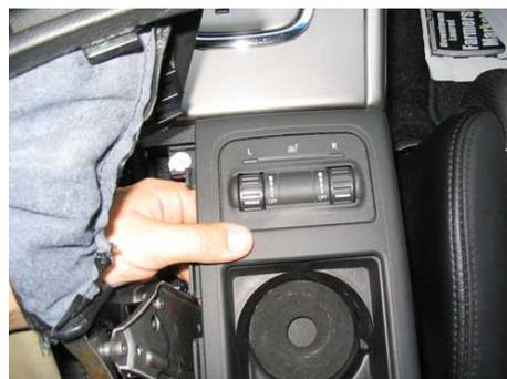
The next steps will vary a bit depending on if you have a manual transmission or an automatic. For manuals, just unscrew the shift knob and pull the shifter boot off. For automatics, place some electrical tape over a flat head screwdriver to prevent scratches and remove the chrome ring around the shifter by gently prying on both sides of the trim with the screwdriver until it comes out.
