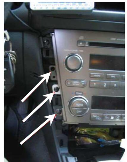
Once the 3 screws on each side of the radio are removed (6 total), the whole radio should come out easily. There are several plugs at the back of the radio to disconnect before you can remove the radio from the car however.
