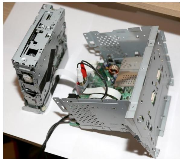
Carefully reassemble the CD changer to the radio taking care not to let the board or cables hit anything. The ribbon cables can also easily be tugged out of contact. Once the CD changer is slid back into place, put the 4 screws back in to secure it in place. To replace the face plate, it's easiest to start by aligning the top and carefully push it back into place until all of the mounting tabs click.
