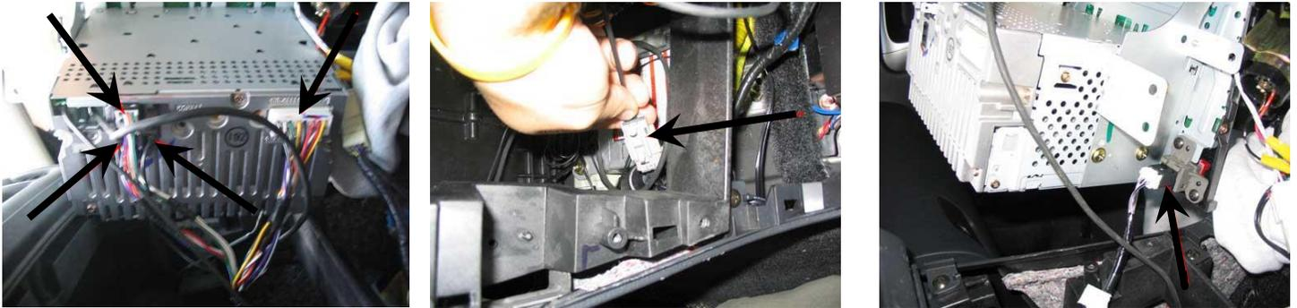
The main radio harness is the big white plug going into the back. There's also a grounding plug, two HVAC plugs, the antenna plug (which is hidden back in the lower left hand side of the radio pocket) and the hazard switch plug.
