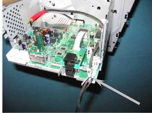
Once the patch cord is prepared, set the radio & changer + board next to each other. Plug the stereo patch cable into the aux port on the accessory board and then plug the 2" ribbon cable into the connector on the radio that the CD changer ribbon was removed from earlier. Again, make sure all the ribbon cables are straight and the aux port is facing the passenger side of the radio.
