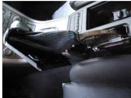
Next, empty the contents of the armrest cubby and remove the carpet on the bottom of the cubby to reveal two mounting screws. Removing these screws will loosen the rear of the armrest, and then only two plastic clips hold the front. Firmly grasping both sides of the front of the armrest and tugging straight up should dislodge both of these clips. It's unnecessary to completely remove the armrest, simply move it back a few inches to better reveal the transmission mount trim.
