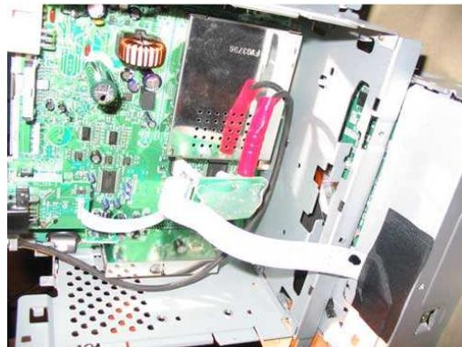
Carefully reassemble the CD changer to the radio taking care not to have the board or cables hit anything. Once the CD changer is slid back into place, put the 4 screws back in to secure it in place. To replace the face plate, it's easiest to start by aligning the top and carefully push it back into place until all of the mounting tabs click.
