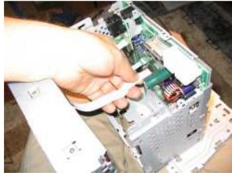
Now the radio is completely disassembled & it's ready to add the accessory board.
