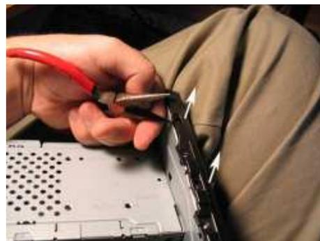
Once the face has been removed, 4 screws are revealed holding the CD changer in place. They are in the middle near the top as indicated with arrows in the picture. Once these are removed, the CD changer should lift out fairly easily. It may be necessary to gently pull on the sides at the back to free the mounting clips of the changer.
