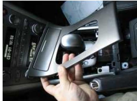
Once this piece of trim is removed, two screws are revealed holding each piece of trim that runs up the length of the radio. Remove these two screws and each piece should simply lift out. The clips holding them in place pop right out as you lift each length of trim, revealing the 6 screws holding the radio in place.
