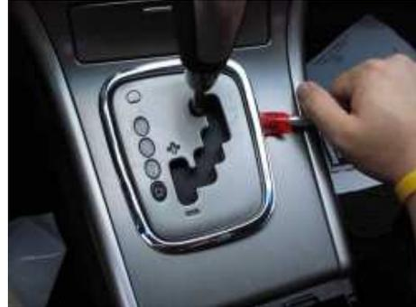
Once the shifter trim is removed, use the same screwdriver to pop up the rear end of the trim surrounding the shifter. Once the back is popped up, the whole thing should lift out. Automatics need to put the key in the ignition & foot on the brake to shift into neutral to remove this part (it is not necessary to turn on the engine). At this point you should lay a towel or old shirt across the trim pieces to help prevent scratches.
